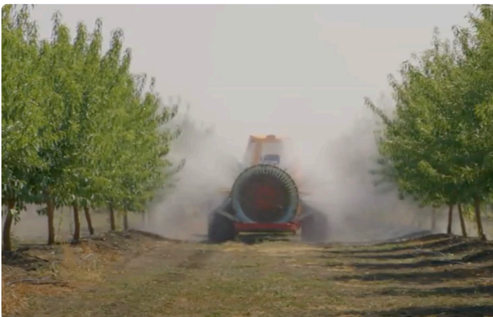
Autonomous AR-500 specialty tractor towing a sprayer
