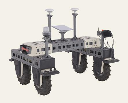
The Amiga Flex bridges the gap between lab and field – a durable test and development platform built for real-world R&D and commercial deployments in outdoor automation.
